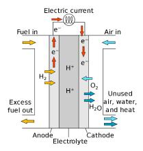
Proton exchange membrane fuel cell process
